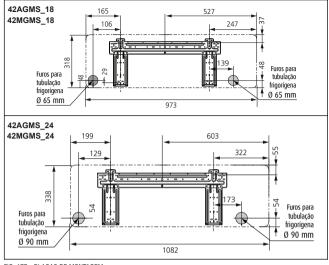
FIG. 17B - PLACAS DE MONTAGEM
