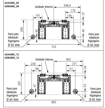
FIG. 17A - PLACAS DE MONTAGEM
